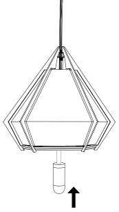
STEP 4 Pass the wires through the stem section with the canopy attached and screw this section onto the top threaded nipple.
