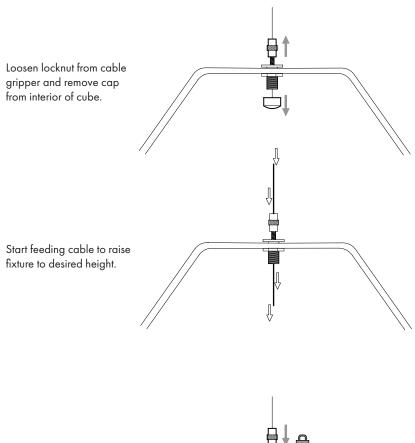
Very tightly secure locknut back in place and cut excess cable before reattaching bottom cap.
