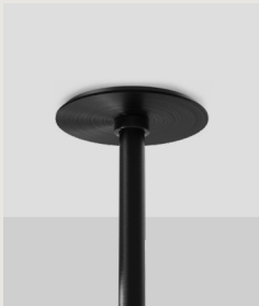
SLIM Ø20MM FIXED CANOPY CAN.SL.F20.X-XXX Ø120 X 7MM / 4.7" X 0.3" DRIVER HOUSED IN CEILING
