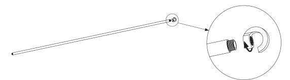
2. Feed the black lead wire (C) up from the fixture through the top of the stem. Attach the stem (A) with connected hub cap (B) to the Astral hub (D) by screwing three screws into place.
