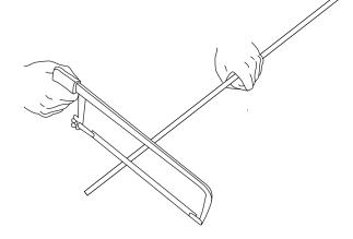
3. Now that the cover tube is cut to 28.5", measure the all thread tube to be 28.5 and 1/2" long. And place a mark, with a marker or tape.
