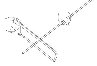
3. Now that the cover tube is cut to 25", measure the all thread tube to be 25 and 1/2" long. And place a mark, with a marker or tape.
