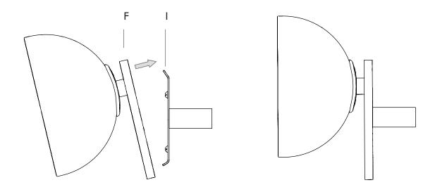
5. Once the fixture assembly is resting in place, use the provided Hex Key (G) to tight the bottom set screw to the crossbar until the backplate is secured.
