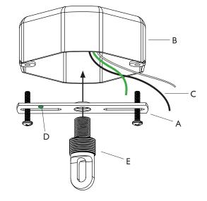
4. Unscrew the hangstraight nut (F) from the hangstraight. Feed onto wire from fixture, followed by the canopy. Carefully raise fixture to ceiling and hold, while guiding the lead wire through the hangstraight into the junction box.
