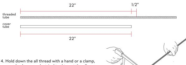
4. Hold down the all thread with a hand or a clamp, use a hacksaw or electrical tool to cut the all thread tube. Recommended to clean all thread tube after cutting to remove any metal chippings.
