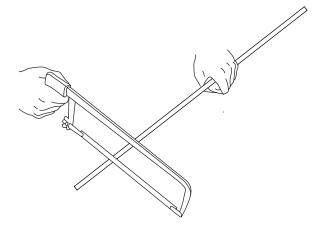
3. Now that the cover tube is cut to 25", measure the all thread tube to be 25 and 1/2" long. And place a mark, with a marker or tape.
