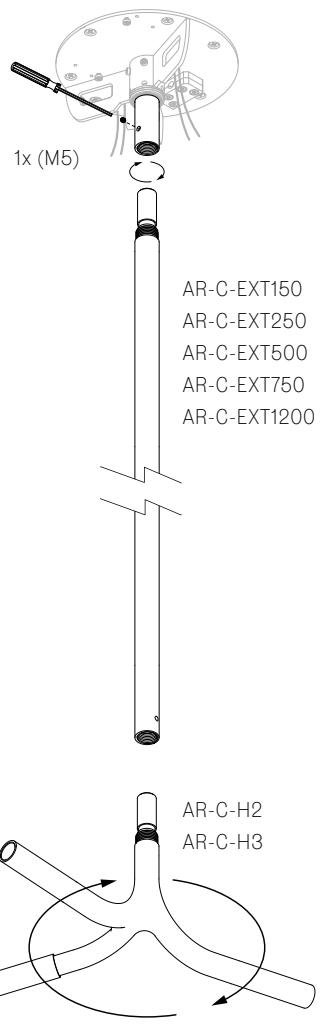
**EN** If the system does not require an extender (AR-C-EXT), then thread the hub (AR-C-H) onto the canopy connector.
