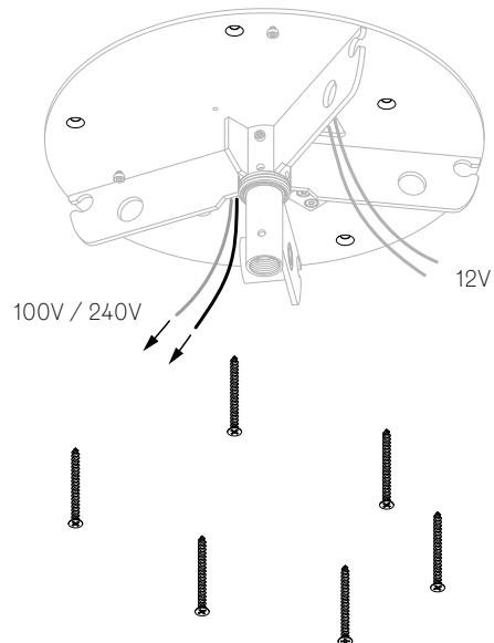
**EN** Use screws provided or substitute equivalent screws to support 36kg load minimum.
