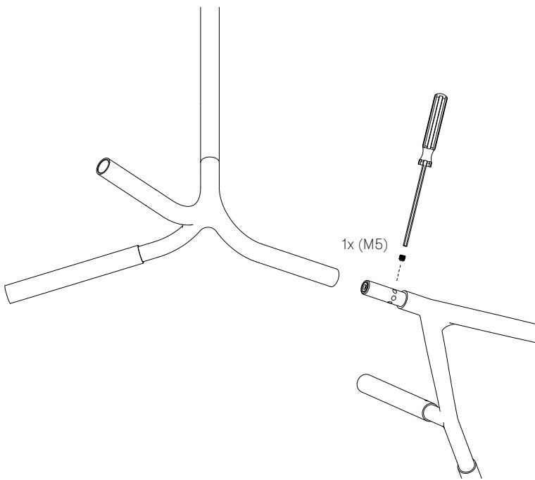
**EN** Attach branches in a balanced manner during installation, one branch across from another. Check the orientation of the branch, adjust if needed. Please reference the drawing on the Pendant Specification Sheet for a visual guide.
