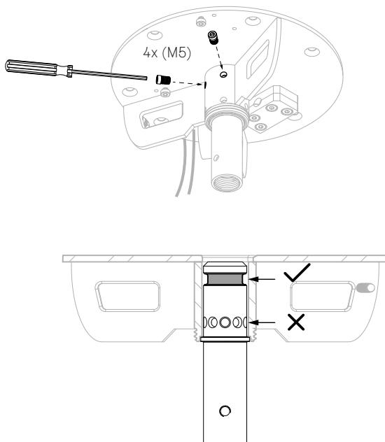
**EN** Attach screws (x4) around circumference of the 1st row of AR-C-CEC. Leave the 2nd row for orientation on step 9.
