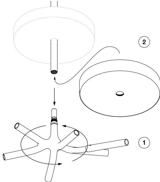
**EN** Remove AR-C-H to add canopy cover, be careful not to scratch the fixture.
