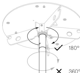
**EN** Check the orientation of the fixture, adjust if needed. Please reference the drawing on the Pendant Specification Sheet for a visual guide.
