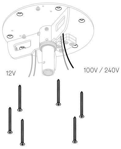
**EN** Use screws provided or substitute equivalent screws to support 36kg load minimum.
