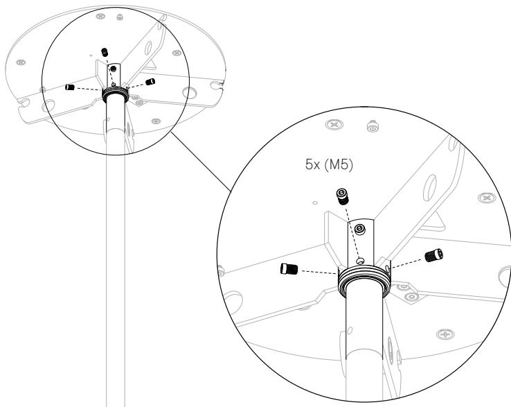
**EN** Tighten screws (x5) on the second row evenly so that all set screws are equally engaged.
