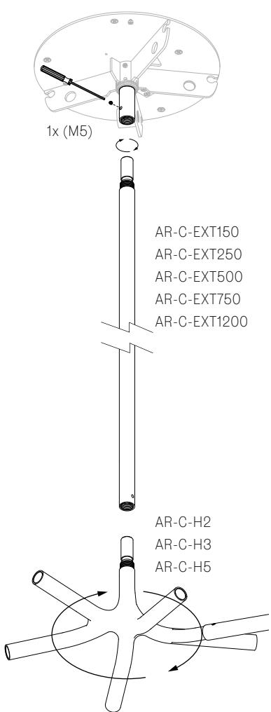
**EN** If the system does not require an extender (AR-C-EXT), then thread the hub (AR-C-H) onto the canopy connector.
