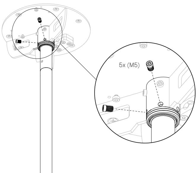
**EN** Tighten screws (x5) on the second row evenly so that all set screws are equally engaged.
