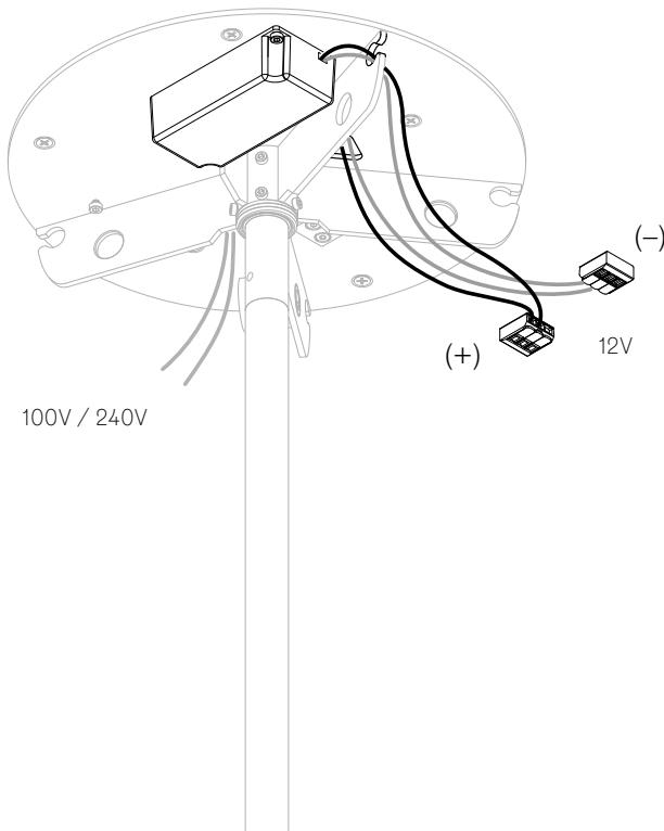
**EN** Connect input low voltage wire to 12V DC output wires by feeding the wires through the slots on the mounting plate.
