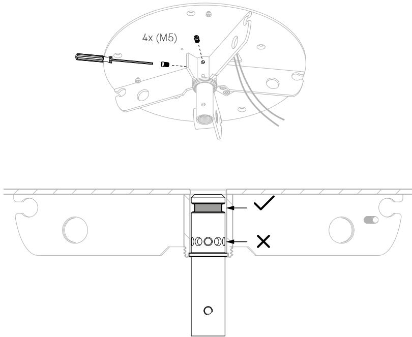
**EN** Attach screws (x4) around circumference of the 1st row of AR-C-CEC. Leave the 2nd row for orientation on step 9.
