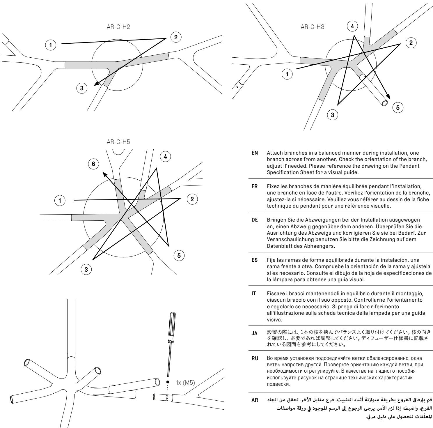
**EN** Attach branches in a balanced manner during installation, one branch across from another. Check the orientation of the branch, adjust if needed. Please reference the drawing on the Pendant Specification Sheet for a visual guide.
