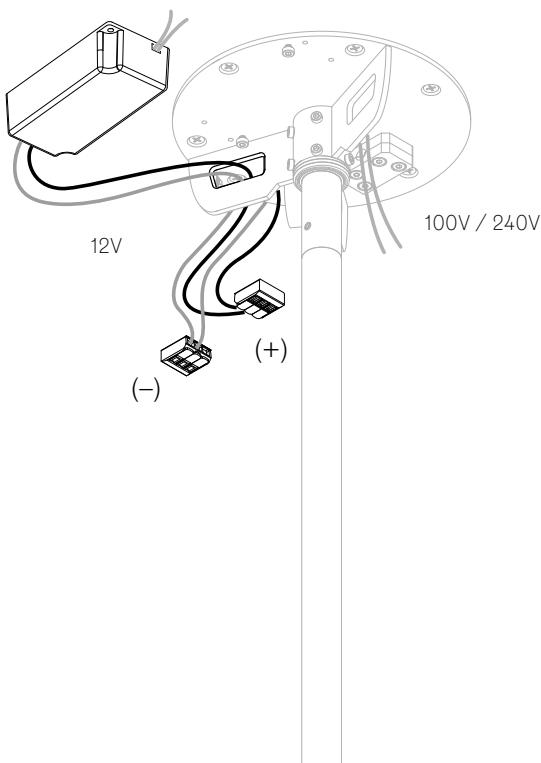
**EN** Connect input low voltage wire to 12V DC output wires by feeding the wires through the slots on the mounting plate.
