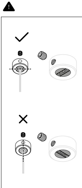
EN Do not overtighten! Perform a gentle tug test to ensure the coaxial cable is secure.
