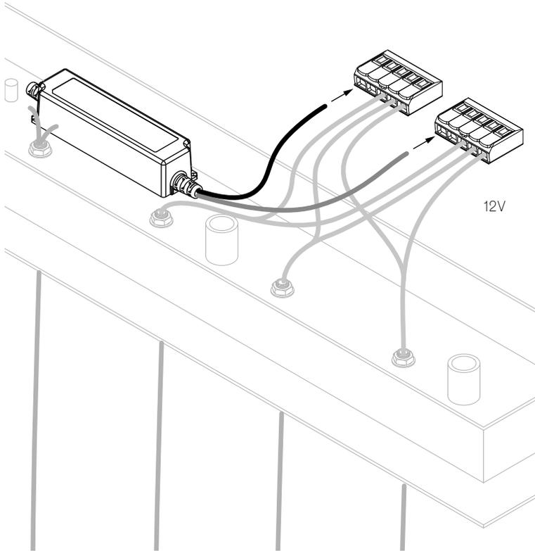
**EN** **LED:** Connect braided wires to negative 12V and insulated wires to positive 12V.
