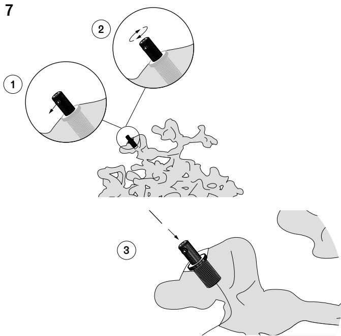
**EN** Bocci recommends wearing gloves during the installation. The aluminum pendant may be sharp to handle. Loosen the set screw and griplock cap located on the pendant that will be connected to a positive cable. Slide the cable through the griplock to set the height.
