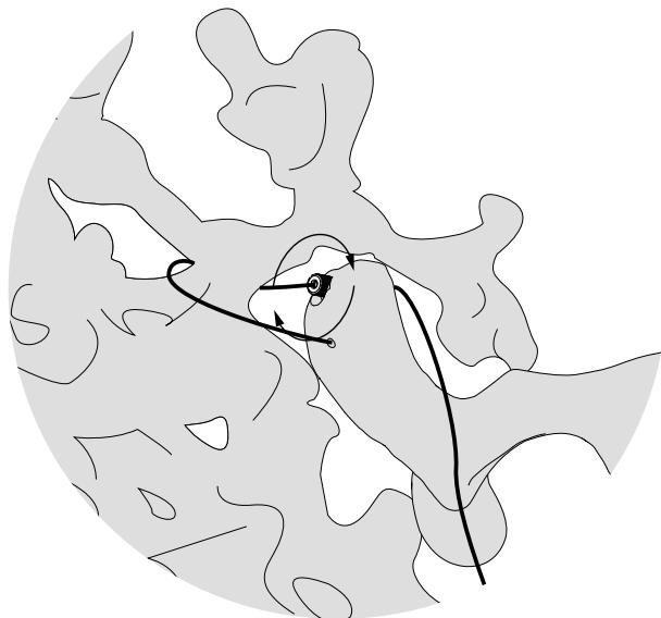
**EN** Tighten the griplock cap to secure the pendant and the lamp assembly.
