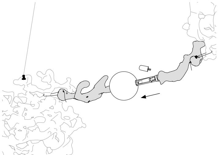
**EN** Unlock the release pin located on the lamp assembly by pushing in with a thin tool.
