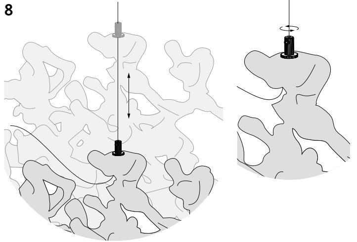
**EN** Repeat these steps for the negative charge pendant and leave the second positive cable until later in the installation. Note: the griplock can be used to adjust and re-adjust the height as necessary; the power will only flow to the pendants when the set screw on the cap is tightened. Only tighten the set screw when the desired height is achieved.
