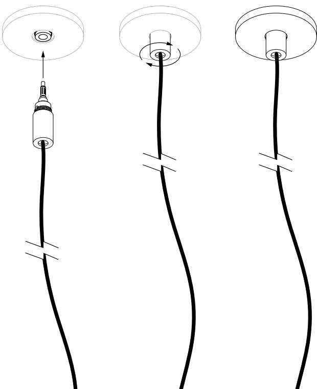
**EN** To avoid kinks, uncoil the coaxial cable in a spool-like manner. Allow the cable to uncoil completely before installing.
