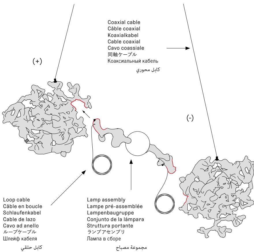
**EN** The lamp assembly must be in contact with the pendants to complete the electrical current that powers the LED.
