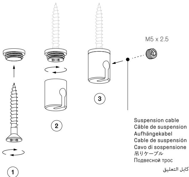
**EN** Once the pendants are suspended and secured, you have the option to add horizontal dimension by using a jacketed suspension cable and pendant anchor kit (included). Ensure adequate structural support for the weight of the pendant, backing may be required.
