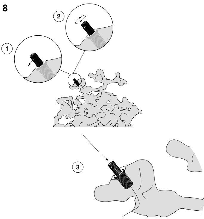
**EN** Bocci recommends wearing gloves during the installation. The aluminum pendant may be sharp to handle. Loosen the set screw and griplock cap located on the pendant that will be connected to a positive cable. Slide the cable through the griplock to set the height.
