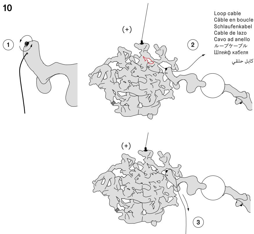
**EN** Find a closed loop on the positive pendant, loosen the griplock cap on the lamp assembly and thread the lamp assembly cable through the pendant.
