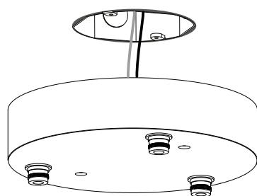
**EN** The client is responsible to ensure junction box is attached to a robust structural substrate.
