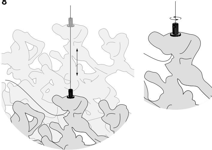
**EN** Repeat these steps for the negative charge pendant and leave the second positive cable until later in the installation. Note: the griplock can be used to adjust and re-adjust the height as necessary; the power will only flow to the pendants when the set screw on the cap is tightened. Only tighten the set screw when the desired height is achieved.
