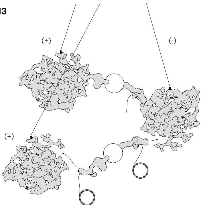
**EN** Repeat these steps to connect the negative pendant. Turn power to fixture on to test the pendant assembly at this stage before moving on to complete the installation. Attach the final pendant to the remaining positive cable and set height and connect the second lamp assembly as per previous steps.
