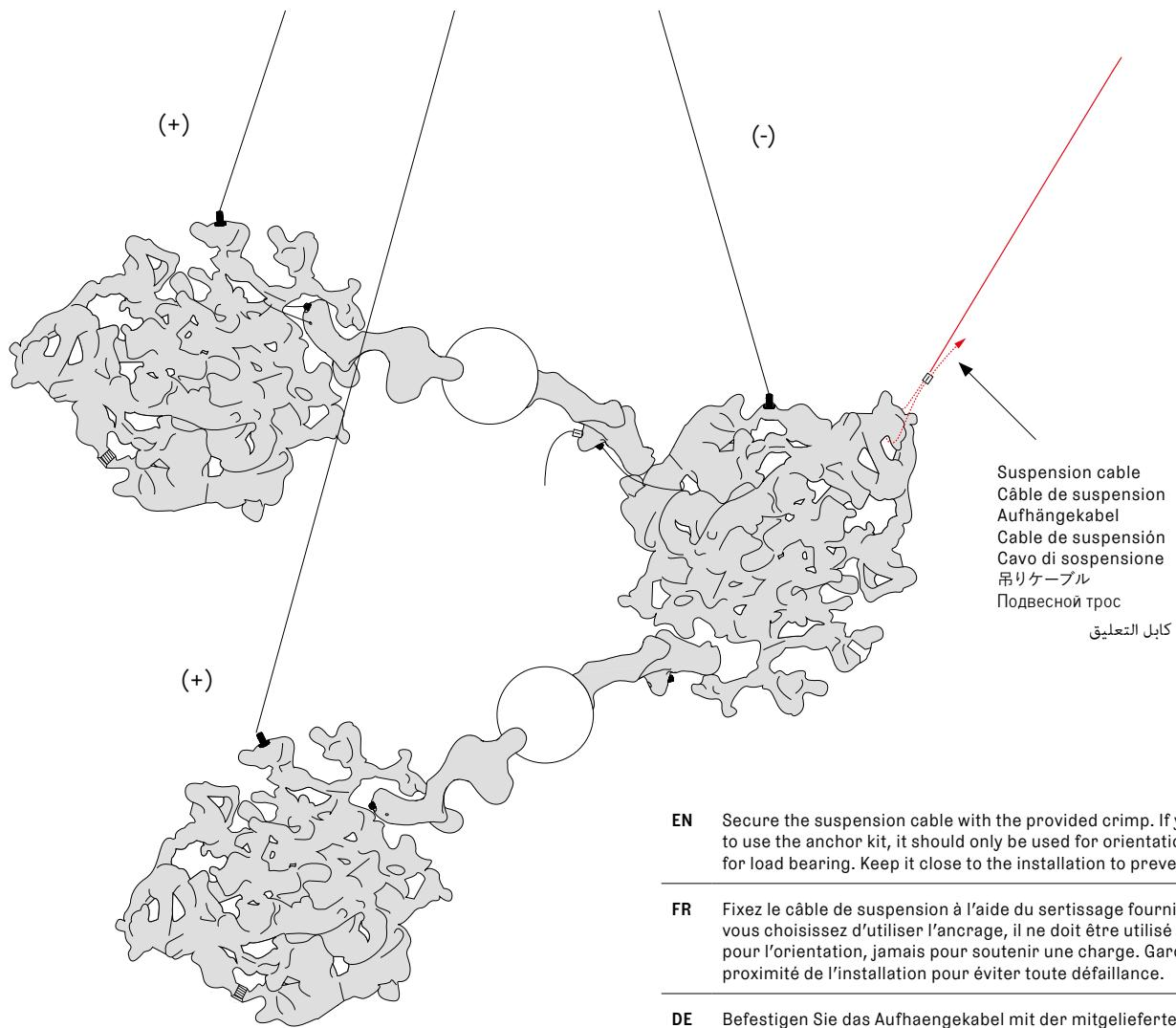
**EN** Secure the suspension cable with the provided crimp. If you choose to use the anchor kit, it should only be used for orientation, never for load bearing. Keep it close to the installation to prevent failure.
