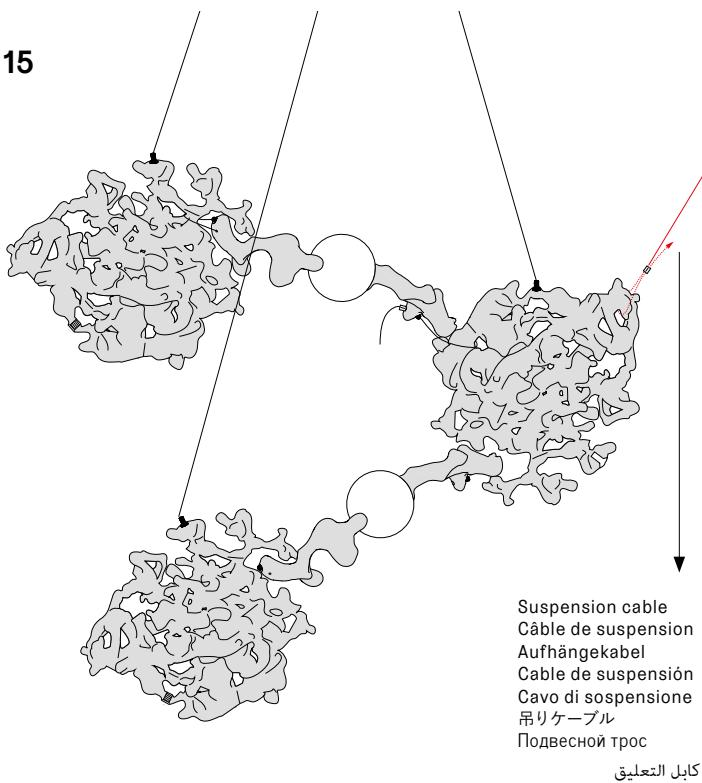
**EN** Secure the suspension cable with the provided crimp. If you choose to use the anchor kit, it should only be used for orientation, never for load bearing. Keep it close to the installation to prevent failure.
