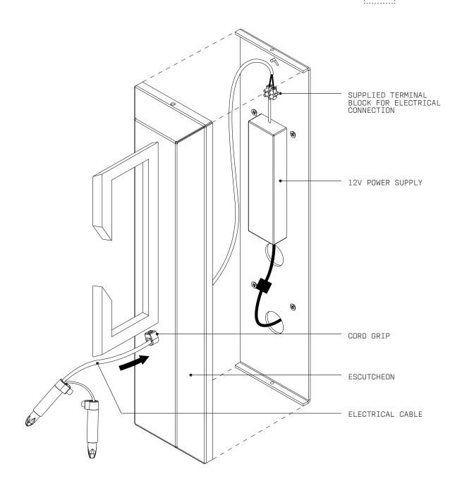
6 Fix brass ESCUTCHEON to BACK PLATE using the supplied fasteners. Leave G4 LAMP ASSEMBLIES resting as they are, these will be placed into the GLASS PURSE in the coming steps.
