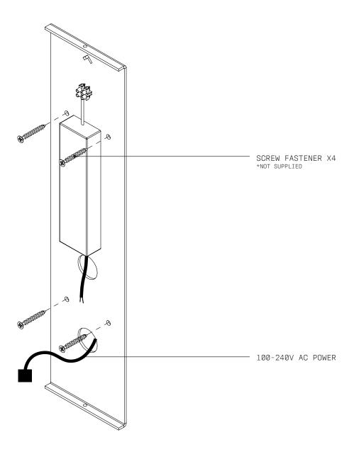
Connect the 110-240V AC POWER to 12V POWER SUPPLY. 4 Refer to supplied WIRING DIAGRAM.  $\rightarrow$
