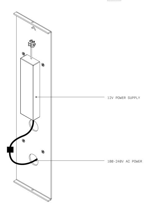
$\frac{5}{-} \qquad \qquad \begin{array}{l} \text{Feed ELECTRICAL CABLE through CORD GRIP in brass ESCUTCHEON. Connect ELECTRICAL} \\ \text{CABLE to 12V POWER SUPPLY.} \end{array}$
