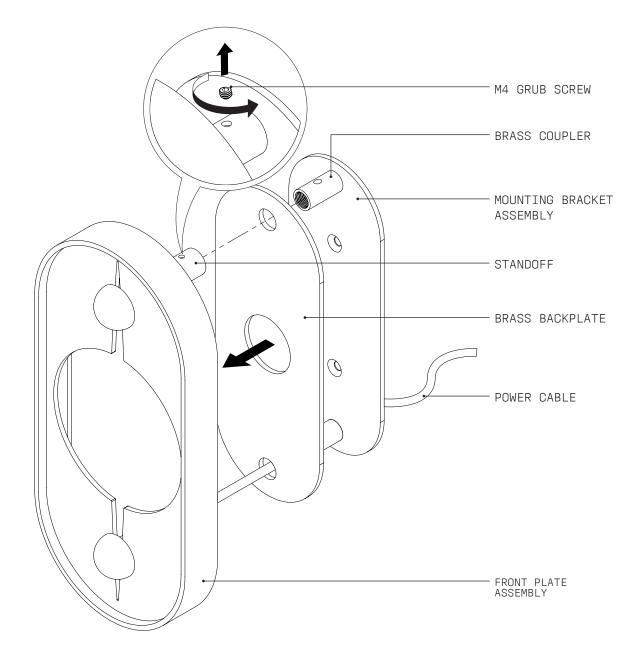
$\frac{2}{-} \qquad \begin{array}{l} \text{Separate the mounting bracket assembly which will be used as a template for sconce installation.} \\ \text{Mark out the two WALL FIXING HOLES and POWER FEED HOLE, as well as a WALL CAVITY location for the power supply.} \\ \end{array}$
