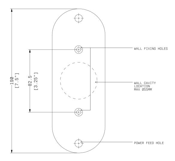
Remove the MOUNTING BRACKET ASSEMBLY and cut the POWER FEED HOLE. 3  $Using \ appropriate \ 2x \ COUNTERSUNK \ SCREW \ FASTENERS, attach \ MOUNTING \ BRACKET \ ASSEMBLY$ to wall substrate.
