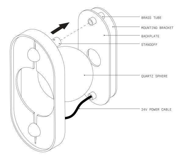
5 Carefully fasten M4 GRUB SCREWS through STANDOFFS, holding the FRONT PLATE ASSEMBLY into position. Ensure M4 GRUB SCREWS sit in small notch on each STANDOFF.
