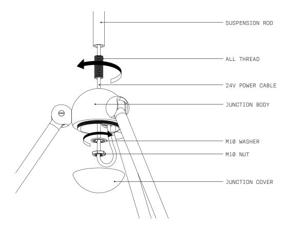
Ensure that the PENDANT is the right way up as per diagram. Feed the 24V DC POWER CABLE and SUSPENSION ROD through their corresponding positions in the escutcheon and the pendant suspension block, as per supplied CANOPY INSTALLATION GUIDE.
