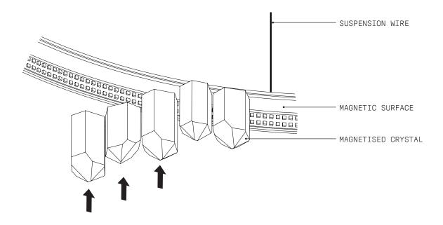
$\frac{7}{2}$  Ensure that the MAGNET on the crystal makes full contact with the MAGNETIC SURFACE on the ring.
