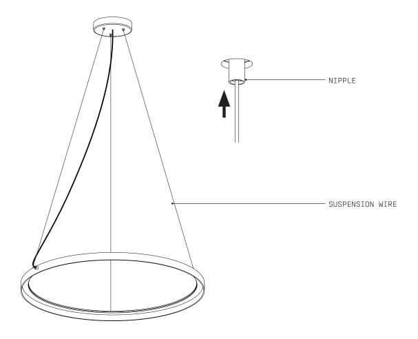
Adjust the level of the fixture using the adjustable CABLE GLIDERS. The lengths of the SUSPENSION WIRES can be adjusted to be lower by taking the weight off the suspension wire, and pushing on the spring loaded NIPPLE on the CABLE GLIDER to release.
