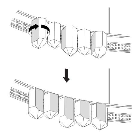
Some MAGNETS are not central to the crystal. Rotate the crystal so each MAGNET sits closest to the
