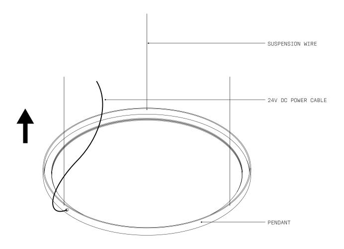
2 Ensure that the PENDANT is the right way up as per diagram and that the SUSPENSION WIRES are not tangled.
