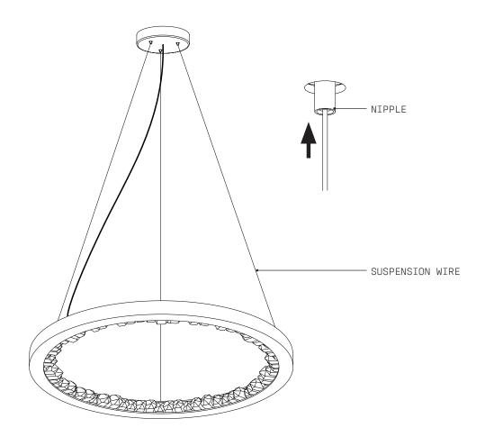
5 Adjust the level of the fixture using the adjustable CABLE GLIDERS. The lengths of the SUSPENSION WIRES can be adjusted to be lower by taking the weight off the suspension wire, and pushing on the spring loaded NIPPLE on the CABLE GLIDER
