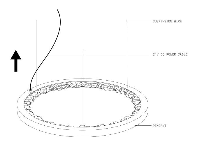
Ensure that the PENDANT is the right way up as per diagram and that the SUSPENSION WIRES are not tangled. Feed the 24V DC POWER CABLE and SUSPENSION WIRES through their corresponding positions in the escutcheon and the pendant suspension block, as per supplied CANOPY INSTALLATION GUIDE.
