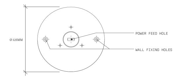
$2 \qquad {\rm Remove \ WALL \ MOUNT \ MODULE \ and \ cut \ POWER \ FEED \ HOLE.}$
