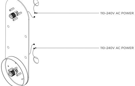
With the electrical connection made, push back wiring into wall cavity and screw fix the sconce backplate to the wall. Ensure the wall fixing fasteners are secured to an adequate load bearing substrate.
