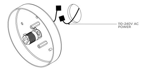
With the electrical connection made, push back wiring into wall cavity and screw fix WALL MOUNT MODULE to the wall. Ensure the wall fixing fasteners are secured to an adequate load bearing substrate.
